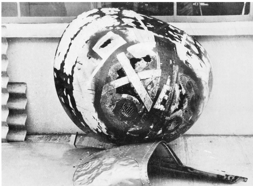
DAMAGE TO NOSE OF AIRCRAFT
