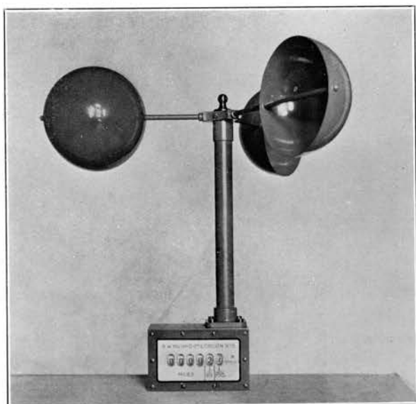
THREE-CUP ANEMOMETER, "RUN OF THE WIND" PATTERN.
