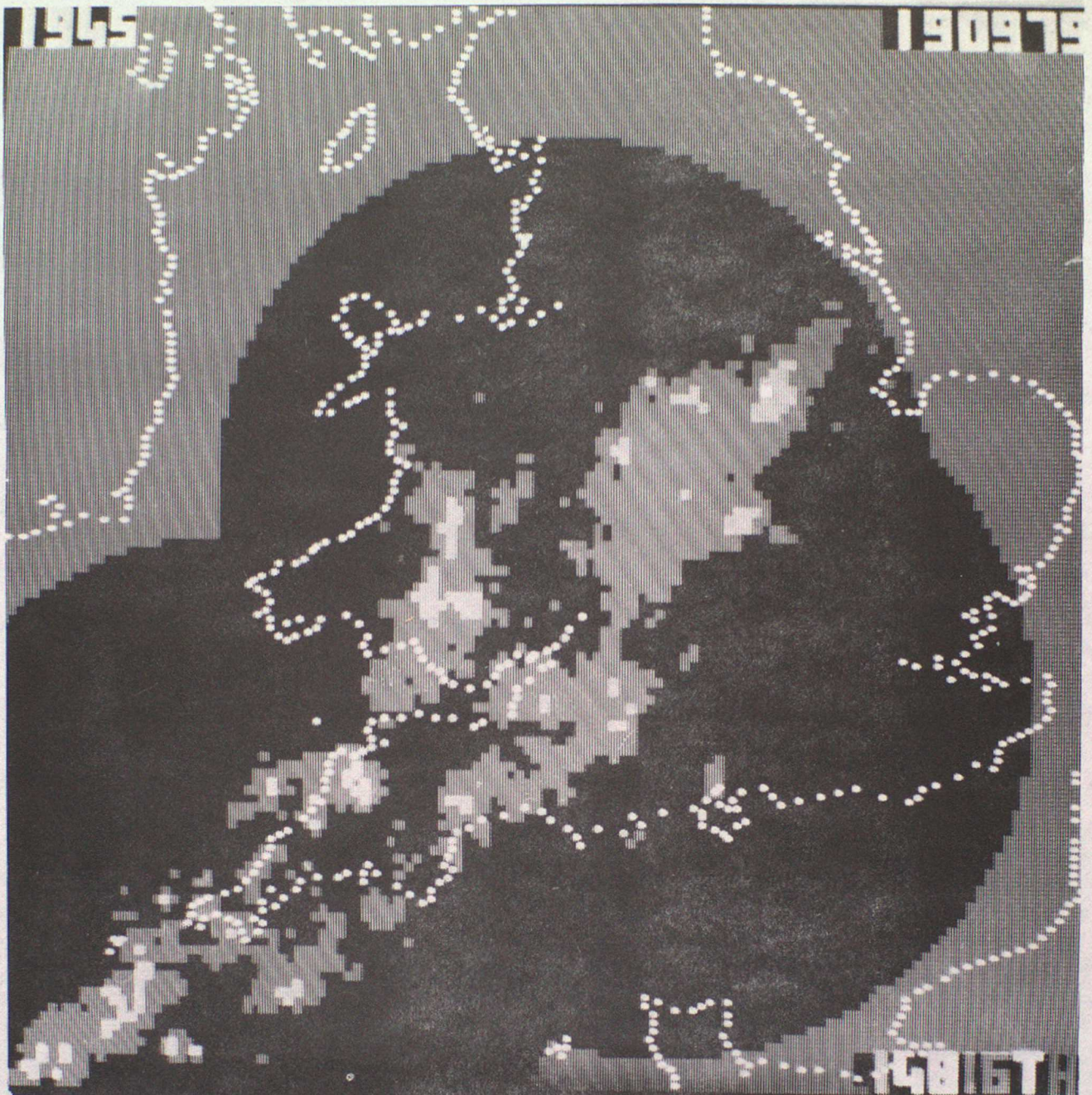
Figure 13(a) Photograph of a composite radar display showing the rainfall distribution in England and Wales at 1945 GMT on 19 September 1979. This composite was generated within 4 min of real-time from data received at Malvern from 3 radars with approximate coverage as indicated by the circles. The display consists of a matrix of 128 \times 128 5 km squares which was displayed on a colour television capable of replaying a sequence of pictures; medium and light grey in the monochrome photograph represent light-to-moderate, and heavy rain, respectively.
