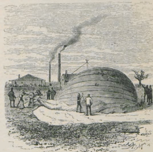
INFLATION OF THE BALLOON WITH A VENTILATOR.
