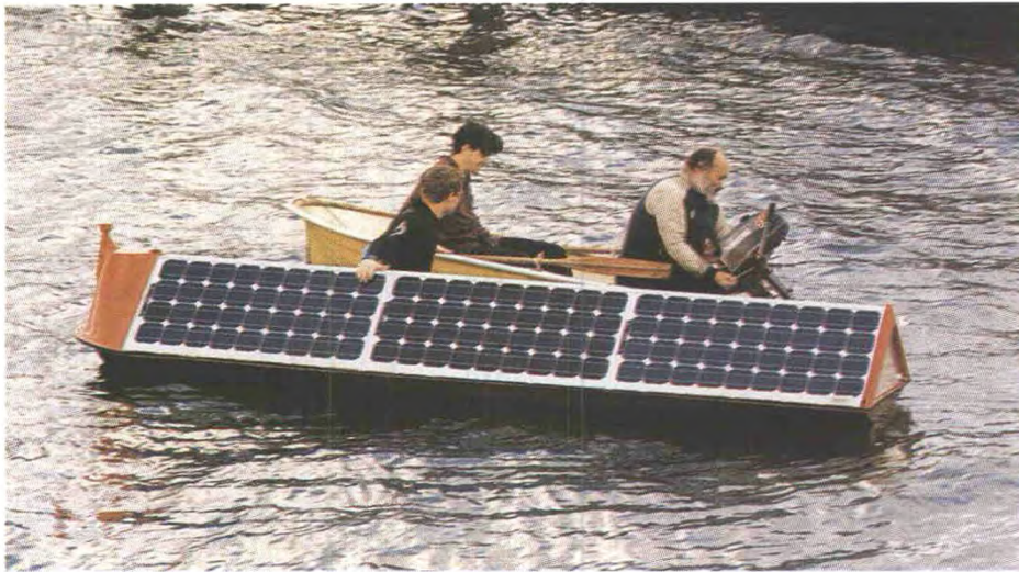
Figure1. The solar electric vessel Goodwill prototype
