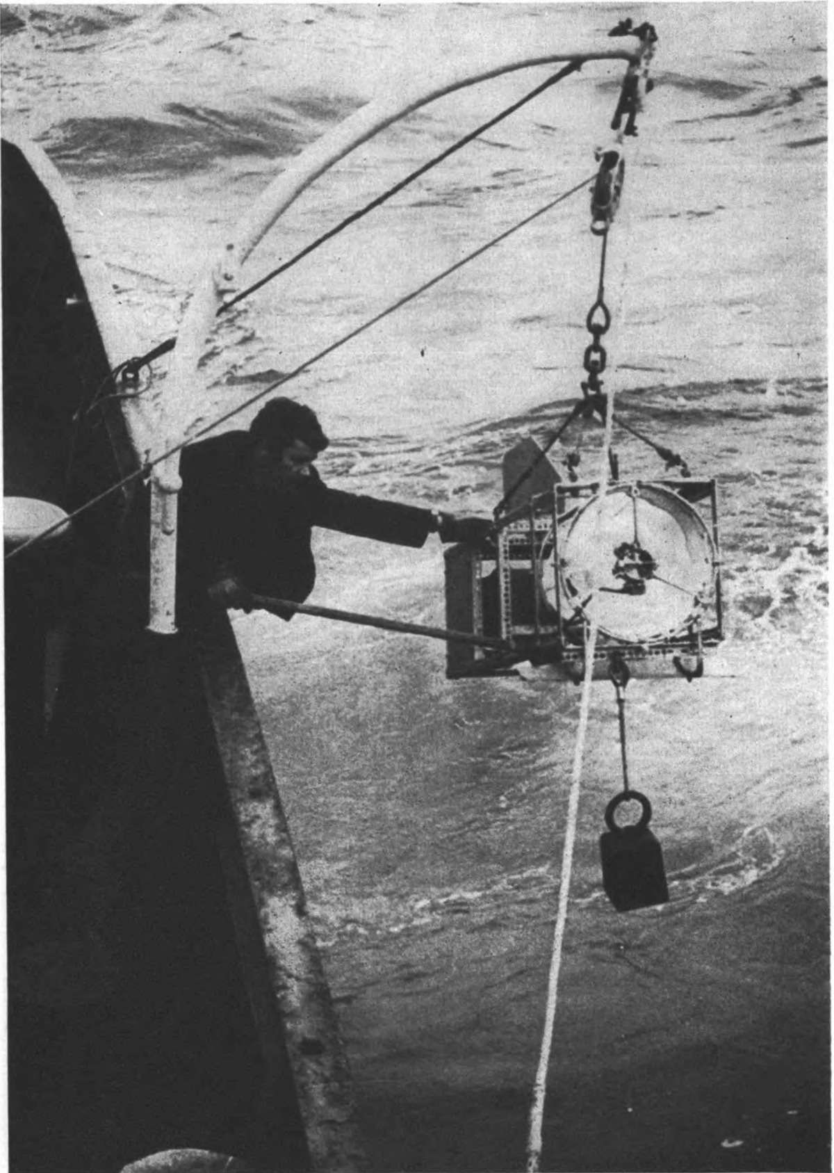
The Longhurst/Hardy Plankton Recorder being launched from an Ocean Weather Ship (see page 76).
