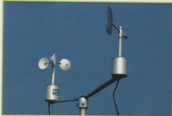
Cup generator anemometer and wind vane
