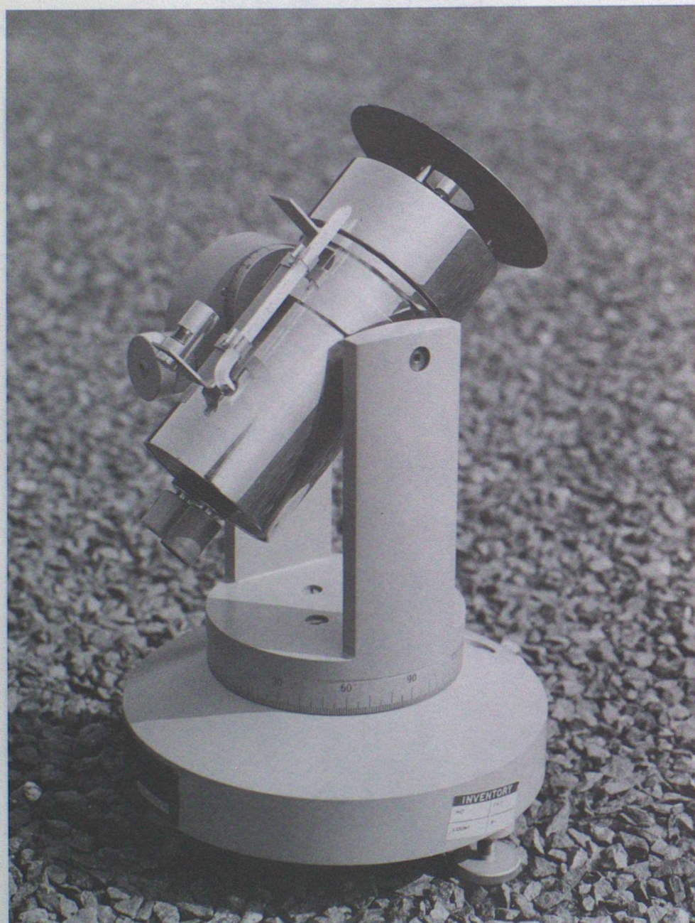
Plate IX. Linke-Fuessner pyrheliometer.
