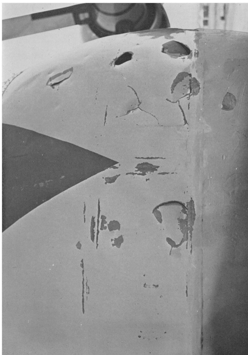
PLATE II—DAMAGE TO NOSE SECTION
