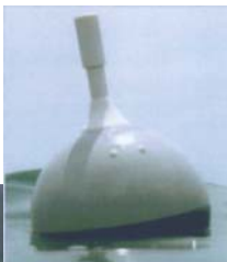
Figure 4(a) (right): SVP-B type buoys afloat and (inset) prior to deployment Note: The buoy shown in the inset is also fitted with a wind vane
