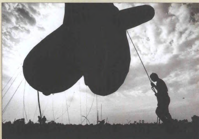
Instruments to monitor wind, temperature and humidity are suspended from tethered balloons up to a mile above ground.
