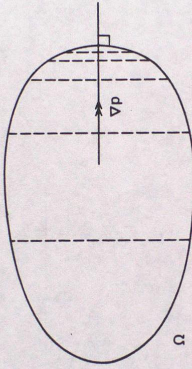
Fig.4 Contours of  $P$  within  $\Omega$ , showing that the extreme value of  $\nabla P$  occurs on the boundary near where  $\nabla P$  is normal to the boundary.
