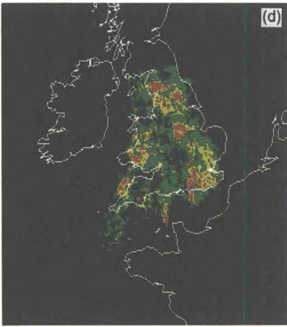
Short-period rainfall forecasts using FRONTIERS. (a) At 1100 GMT on 26 February an area of rain (indicated by the black dots) is crossing the UK from west to east. (b) The rainfall detected by the radar network at 1130 GMT. A forecaster uses the FRONTIERS interactive display to interpret the radar rainfall data in the light of other observations and his understanding of the meteorological situation. The irregular yellow boundary shows the effective area of radar coverage. (c) The forecaster uses cloud images from Meteosat to estimate the likely distribution of rain beyond the range of the radius. FRONTIERS then computes a sequence of forecasts by moving segments of the rainfall pattern at speeds inferred from past motions. This figure shows the forecast for 1430 GMT, 3 hours ahead, in which rainfall deduced from satellite data (shown in white) and from radar measurements are combined. (d) The rainfall pattern measured at 1430 GMT for comparison with the forecast — only rain within the range of values is shown.
