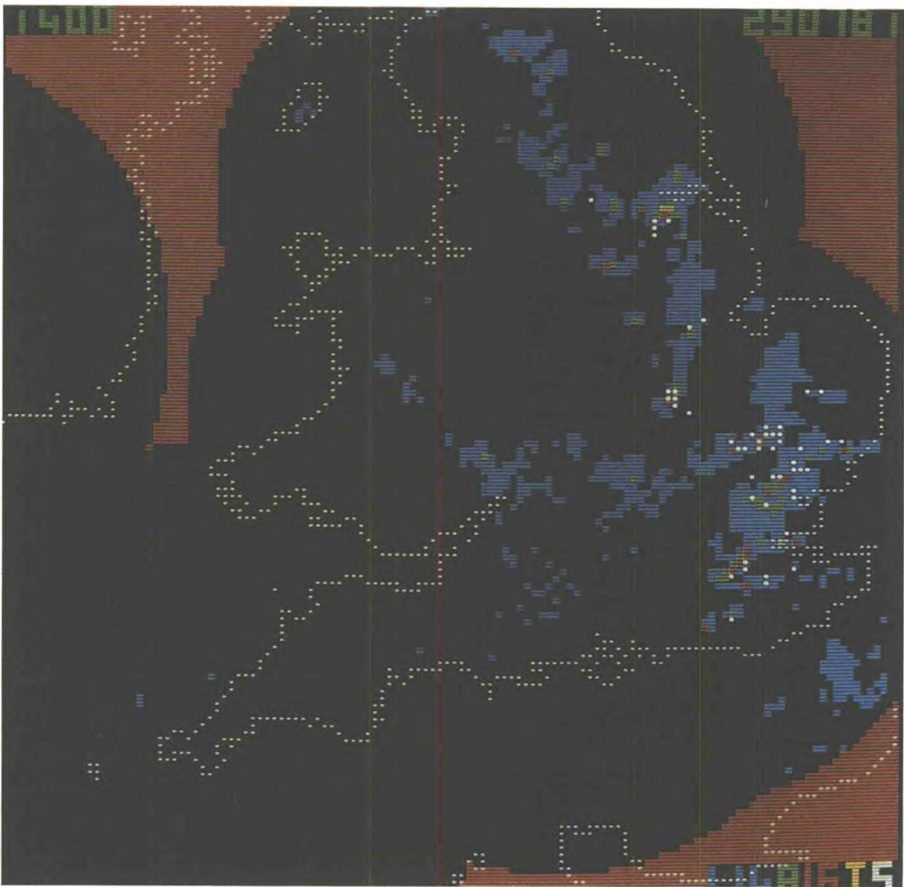
The network display for 1400 GMT on 29 July. The small white dots indicate the lightning strikes detected by the ATD system during the previous 30 minutes. The colours of individual 5 km squares are indicative of the observed rainfall rate.
