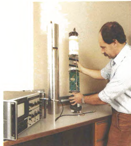
The dropsonde deployed by the Hercules to obtain profiles of wind, temperature and humidity
