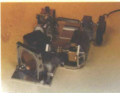
A development-model microwave receiver for the AMSU-B instrument
